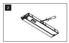
Disengage adapter plate by loosening screw.
