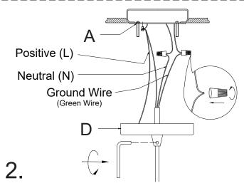
Adjust wire length to desired mounting height, and tighten strain relief screws to secure. Wire fixture to wires in outlet box. Green wire is for Ground.
