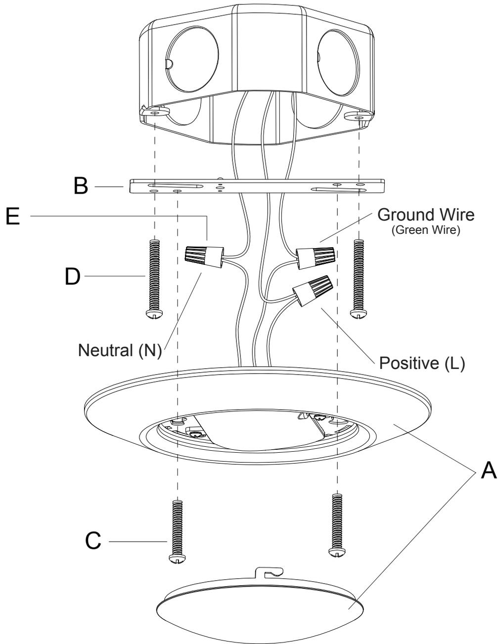
1. Prior to installation, install the mounting bracket on the junction box with mounting screws. Drive screws completely to the end of the junction box.
