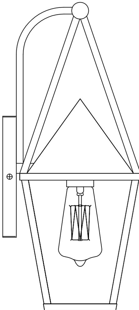
**Lamping | Ampoule: " [1] x[E26 Medium] [60W] (Not Included) "**
