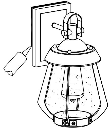
For outdoor use, caulk around fixture with silicone sealant to prevent water intrusion. Leave a gap at the bottom to allow moisture to escape.
