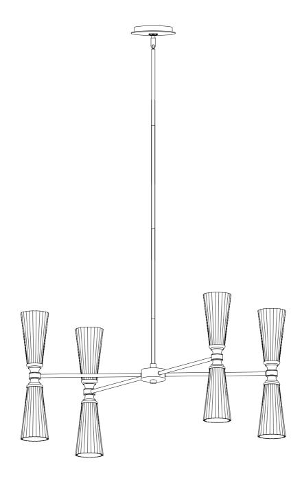
Lamping | Ampoule: 8 x E12 60W ( Not Included )
