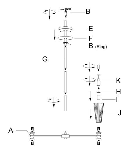
1. Run wire through stems and combine stem lengths to meet desired mounting height.
