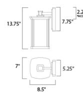
height from center of outlet to top of the fixture
