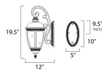
\*height from the top of the fixture to the center of the outlet
