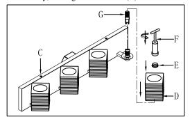
Step.4: Install G9 LED bulb(G) into socket, Position Glass(D) onto the socket of fixture body(C), then secure with socket ring(E) with Glass (D) onto Fixture body(C) by using spanner(F).
