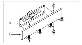
Step.3: Place the fixture body(B) against mounting bracket, Align the two holes of the mounting bracket and fixture body, then tighten the screws(C).
