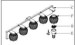
Step.4: Position Glass(F) onto the socket of fixture body(C), then secure with socket ring(D) with Glass (F) onto Fixture body(C) by using spanner(E).
