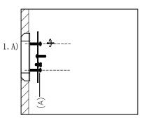
Step.1 Remove mounting bracket from fixture and install to electrical box.
