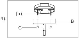
Step.4: Raise canopy (B) over screws (a) and secure with finials (C). Install light bulb. Place glass (H) over the socket, and then secure glass with screw (G).
