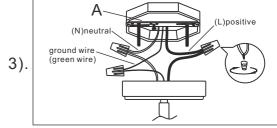
Step.3: Wire fixture to wires in junction box. Copper wire is for Ground.
