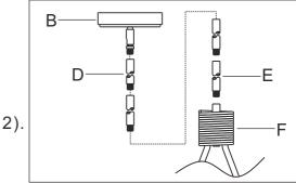
Step.2: Slip first stem section (E) along wire and thread into top of main fixture body (F). Repeat for assembly stem (D) and canopy (B).
