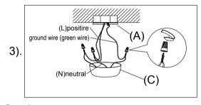
Step.3: Wire fixture to wires in outlet box. Green wire is for Ground.
