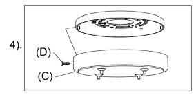
Step.4: Install body (B) to Mounting Strap (A) and tighten Screw (D) through the hole of canopy (C) on the Mounting Strap (A). Place the Candle tube(F) over the socket and Install light bulb.Install the crystal (G) on the lamp body
