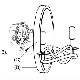
Step.3: Install body (B) to the outlet box and secure with screw(C). Place the Candle tube(D) over the socket and Install light bulb.Install the crystal (E) on the lamp body
