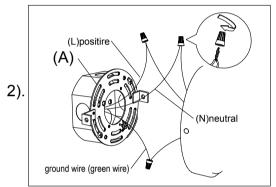
Step.2: Wire fixture to wires in outlet box. Green wire is for Ground.
