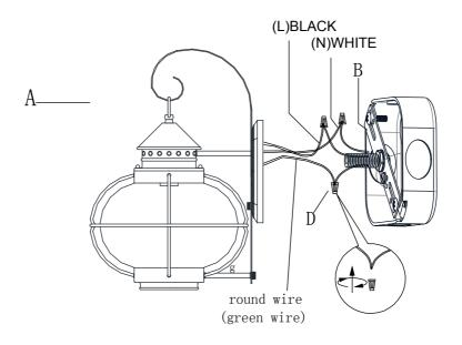
$2.\,$  Caulk around backplate where fixture meets the wall leave a hole at the bottom to allow water to escape.
