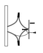
1.Remove mounting bracket from fixture and install to electrical box. Then wire fixture to wires in outlet box. Copper wire is for Ground.
