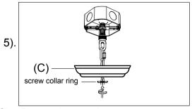
Step.5: Raise Canopy (C) to ceiling and secure with screw collar ring.
