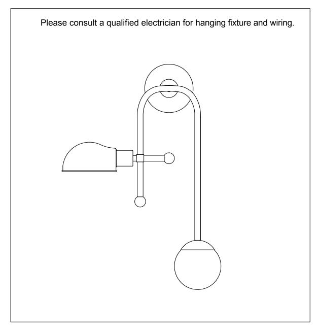
Bulb (included): 1\*4W G9\*LED Bulb + 1\*9W E26\*LED Bulb Bulb (Max wattage): 1\*25W G9 Bulb + 1\*40W E26 Bulb IMPORTANT: Turn off the power at the main fuse or circuit breaker box before starting installation
