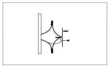
1.Remove mounting bracket from fixture and install to electrical box. Then wire fixture to wires in outlet box. Copper wire is for Ground.
